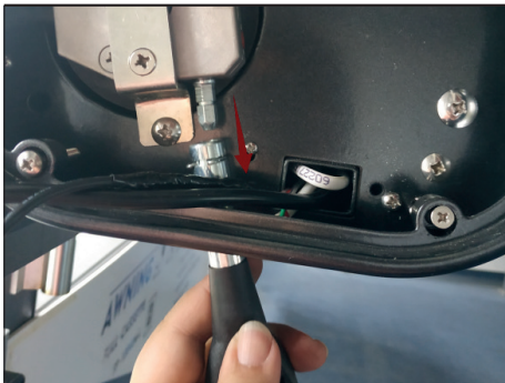
7. Remove the circlip from the crank eyelet and pull out the crank eyelet.
