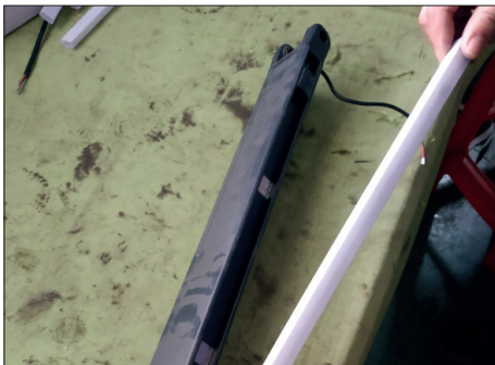
4. Gently pull the LED light tubes out of the long beams.
