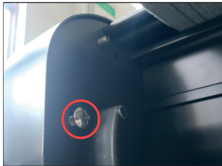
5. Use a screwdriver to loosen the decorative cover screws.
