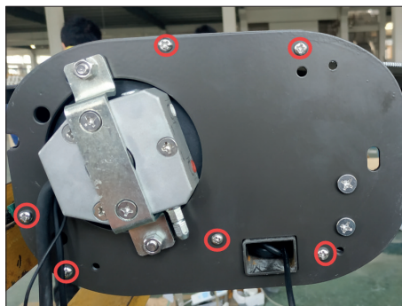
11. Screw out the screws fixing the inner cover.
