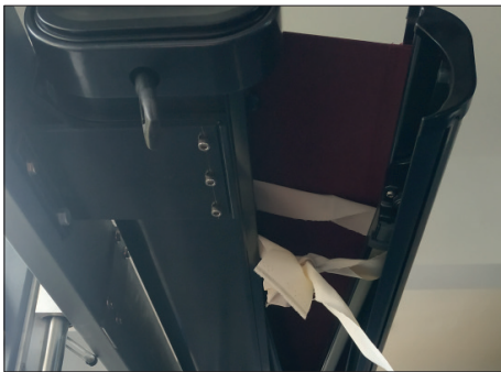
4. Secure the spring-loaded arms tightly with straps to prevent them from bursting open.
