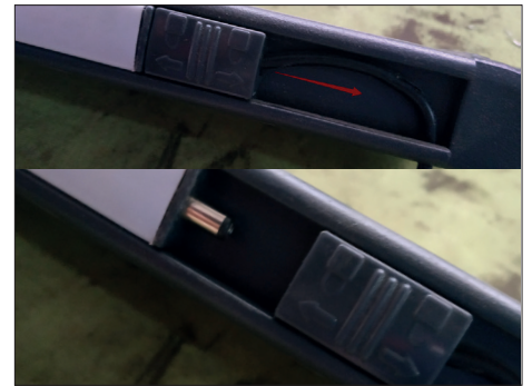
3. Open the LED latch of the longer beams close to the cassette.
