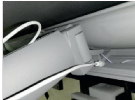
**3.** Unplug the connectors of the LED strips from the shoulder bracket.
