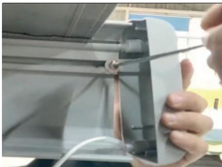
**8.** Remove the side caps of the left and right front bar.
