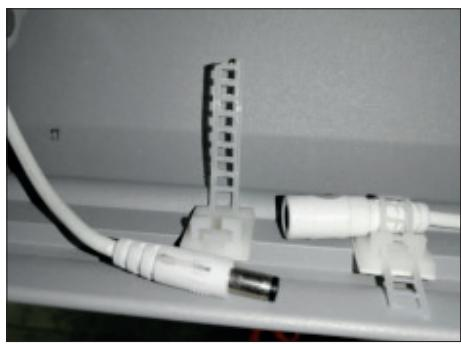
**4.** Open the wire holders of the LED strips in the arms, then unplug the connectors of the LED strips and the one in the front bar.
