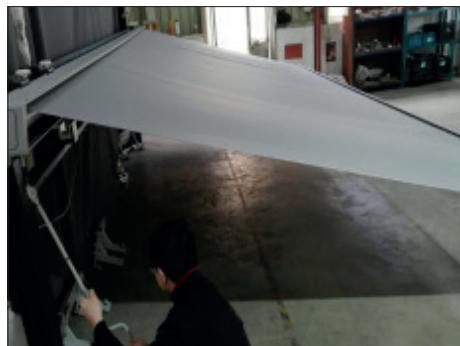
**1.** Turn off the power and use hand crank to open the awning.
