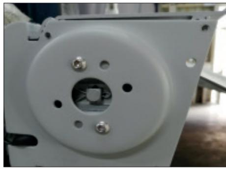
**4.** Use a screwdriver to pick off the screws of hood locking plate.
