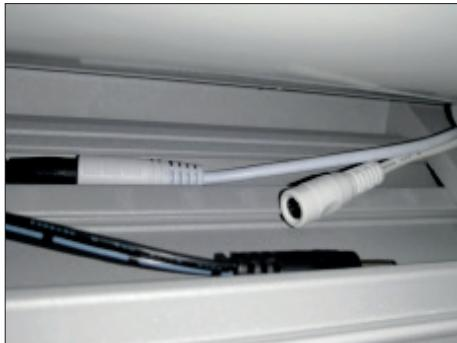
**2.** Unplug the wire connectors inside the hood and the LED strips in the arms.
