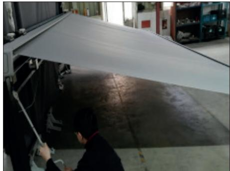
**1.** Turn off power and use hand crank to open the awning, or turn power off after opening the awning electrically.
