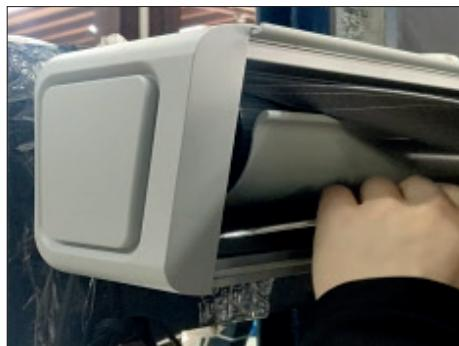
**2.** Use a 4# Allen wrench to remove the screws of hood side cap.
