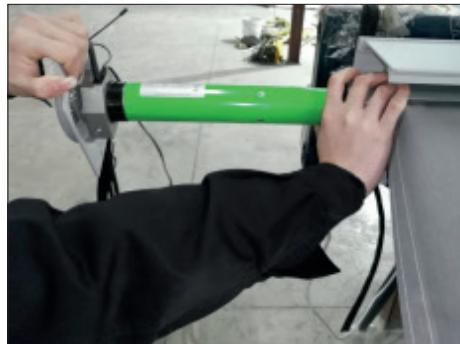
**7.** Pull the motor and the hood locking plate out of the roller tube.
