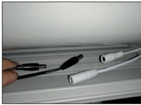
**5.** Separate the connector of the LED strip and the one of the motor.
