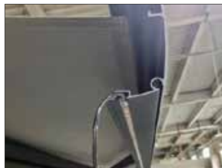
9. Take the LED strip out of the LED holder in the front bar.
