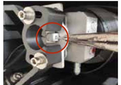
6. Pull the cotter pin out with pliers.
