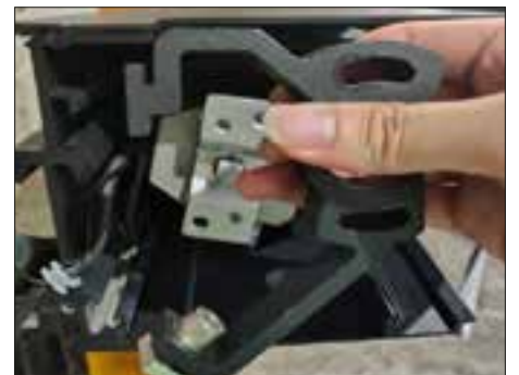
9. Remove the roller bracket.
