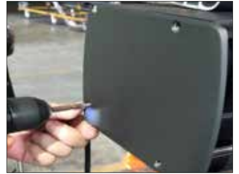
3. Loosen the screws on the hood side cap.
