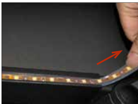
7. Pull the LED strips out of the arms.
