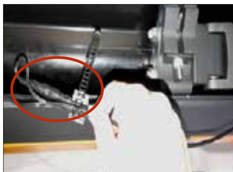
5. Separate the connectors between the LED strip and the motor.
