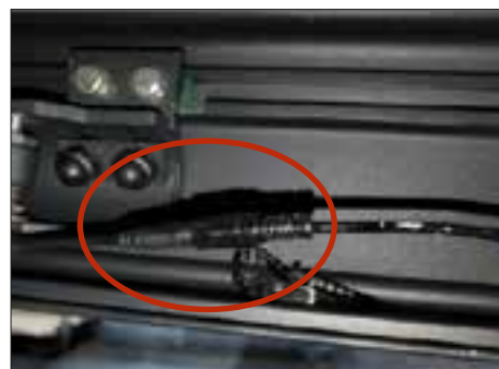
6. Open the wire holders of the LED strip connectors inside the arm, and separate the connectors.
