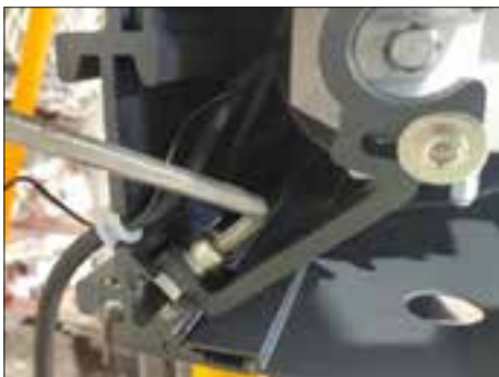
7. Use a 6# hex wrench to loosen the screw as shown above.
