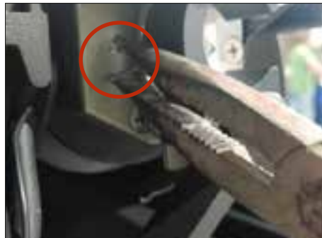
5. Use pliers to close the ends of the cotter pin in the motor holder.
