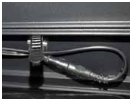
11. Separate the LED line from the awning power line.
