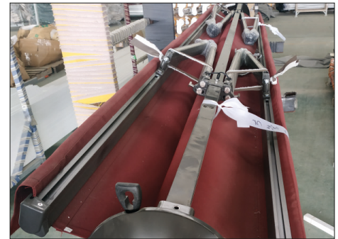
6. Loosen the motor lifting ring and open a little cloth.
