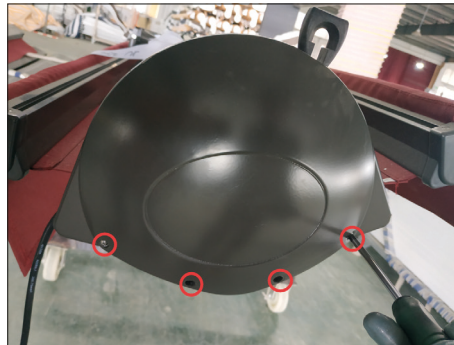
8. Screw out the cross-head screws of the end cover at the motor end.
