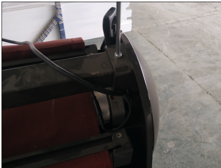
7. Loosen the end cap screws with an Allen wrench.
