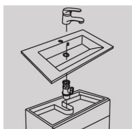
The counter top must be compatible with the furniture unit (installation of siphons and plugholes).
