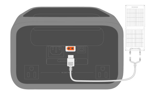
The solar charging cable (solar to XT60i charging cable) and the solar panel are not included in the package.
