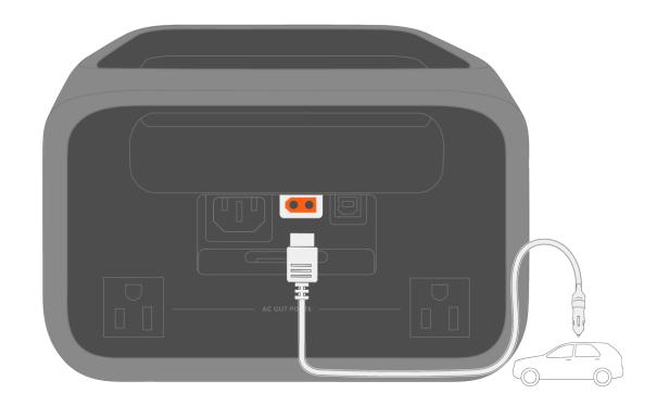
To avoid failure to start the vehicle due to insufficient car battery, start the vehicle first before you begin car charging. In addition, make sure that the car charging cable is securely connected to the cigarette lighter socket.
