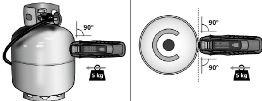
Place the measuring head vertically on the surface of the cylinder and press it down in this position.
