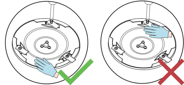
4. Install and ensure the new blades and screws are securely fastened (Torque: 1 N·m).
