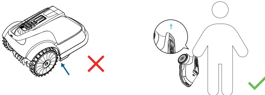
**WARNING :** Never lift or carry the mower while its motor is operating or rotating.
