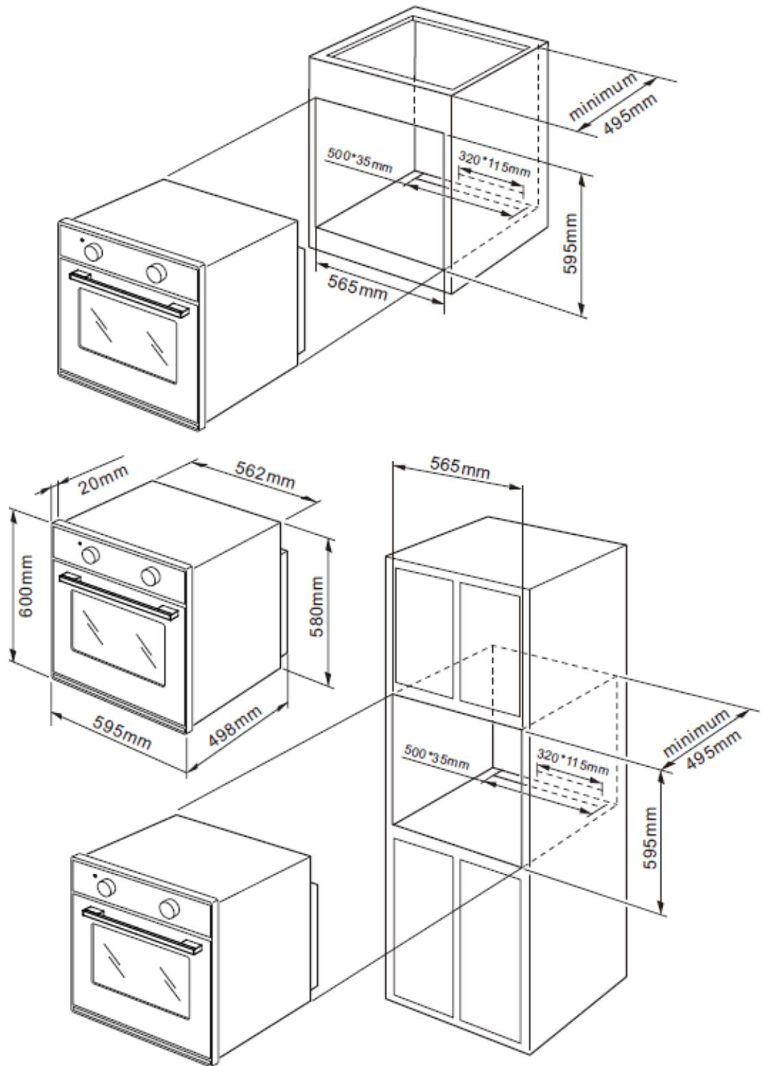
FIG. 2: HOW TO FIX THE OVEN
