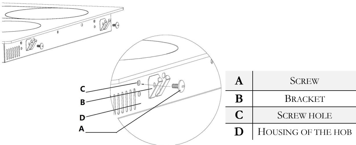
3. Insert the hob into the installation opening and align it correctly. Push the hob down carefully until the hob and the seal are in firm contact to the worktop (s. fig. below).
