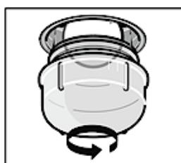
4. Unscrew the illuminant from the socket (s. fig. below) and replace it with a high temperature illuminant (300 °C) of the **same type**: Voltage 230 V / Power 25 W. Do not use any other type of illuminant.
