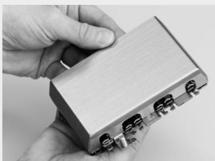
After connecting the data cable, replace the enclosure cover starting with the centering aid (7) directly behind the retaining tab (3).
