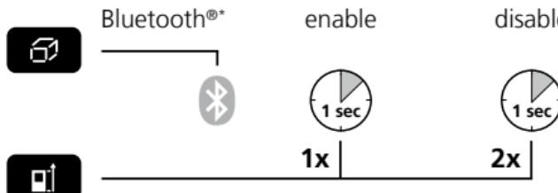
When enabled the Bluetooth®\* symbol appears on the display (g). When the function is active, a mobile device can connect by means of an app to the measuring device.
