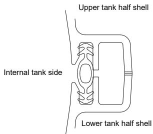
In order to connect the shells, the quick connectors are attached in an alternating manner to the left and to the right. For this, every second connector is pre-adjusted manually in the first step and afterwards attached using a hammer and a wooden support. In order to facilitate the installation, the connectors should be greased on the inner edges. The connectors engage in their final position.
