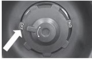
5. Move the tank cap vent lever to the "OFF" position.
