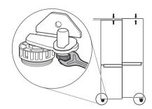
1 Open the door and use the spanner 1 to loosen the keeper nut by turning it to the left.
