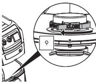
Turn the red rotary switch (on the inside of the suction opening) until the stop: the text "CLOSE" shows upwards to the marking ▲.
