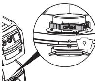
Turn the red rotary switch (on the inside of the suction opening) to the stop: the text "OPEN" shows upwards to the marking ▲.
