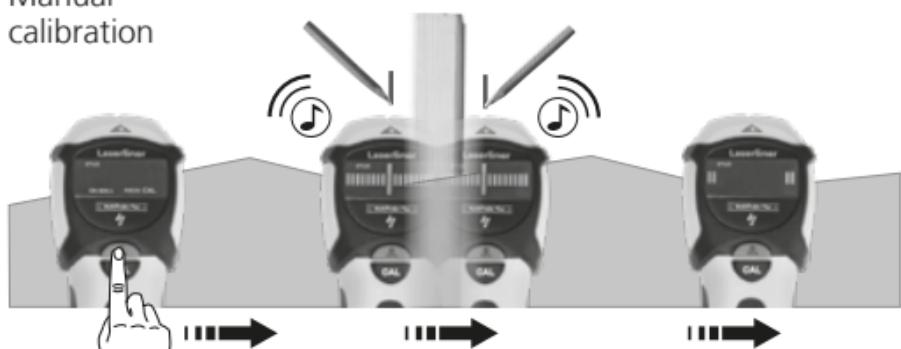
Tip 1: The position between the two markings is the mid-point of the stud.
