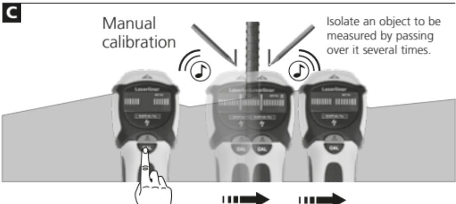
Tip 1: The position between the two markings is the mid-point of the metal object. Through the high measuring sensitivity, thick metal objects appear broader than they are in real life. Therefore move the device over the newly found object as shown in Image B. The device is calibrated automatically during this process. Manual calibration should be performed near the place found last as shown in Image C. Repeat this step as needed.
