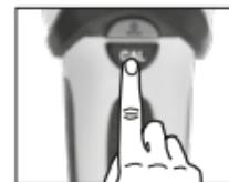
Maximum sensitivity is achieved when the device is held in the air while calibrating. This can be useful for METAL and AC-SCAN measurements.
