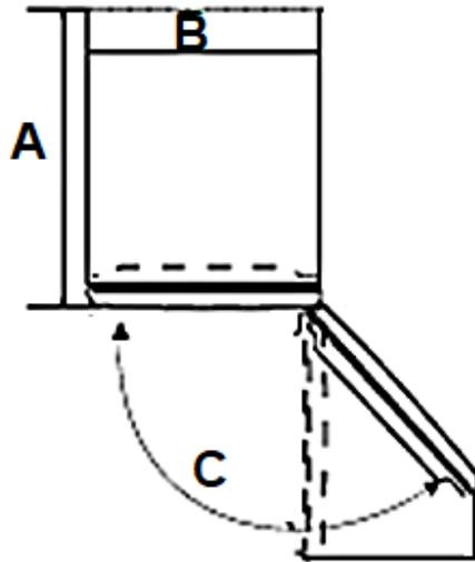
**A = DEPTH / B = WIDTH / C = DOOR OPENING ANGLE**
