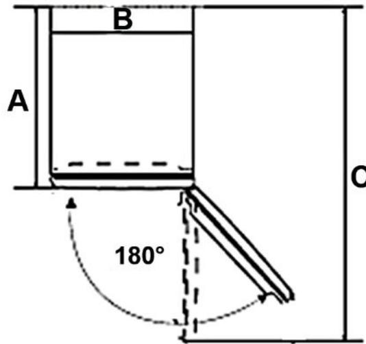
A = DEPTH / B = WIDTH / C = DEPTH (WHEN THE DOOR IS OPEN)
