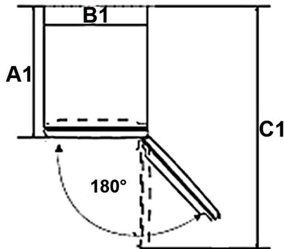
A 1 = Depth / B 1 = Width / C 1 = Depth (when the door is open)
