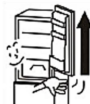
3. Unscrew the middle hinge (C). Remove the door.
