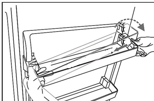
**i** The door trays can be removed and installed for cleaning as shown above.
