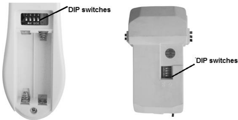
Fig. 8 Remote battery compartment
