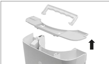
Dismount the water tank for cleaning and remount it in the reverse way before reinstalling it to the appliance
