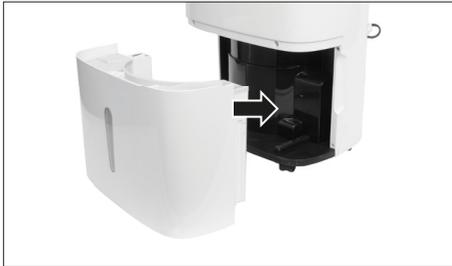
Empty and reinstall the water tank **4**. Make sure it is installed properly.
