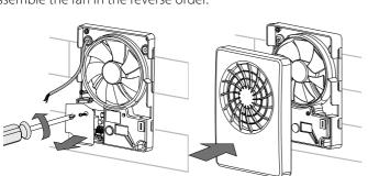
6. Fix the fan with the screws.
