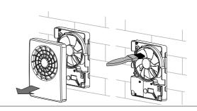
3. Wash the front panel under running water. Wipe the front panel surface dry.
