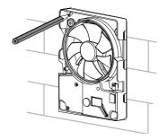
5. Lead the power cable to the ventilation hole, drill the mounting holes and install the dowels.
