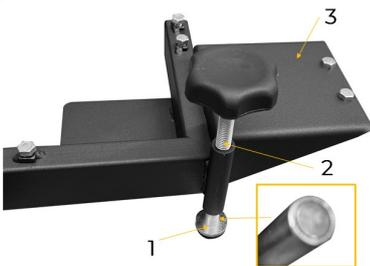
Fit the stopper (1) to the corner connector (3) with the swivel castors. To do this, put the stopper (1) into the tube and screw in the bolt (2) from the top.
