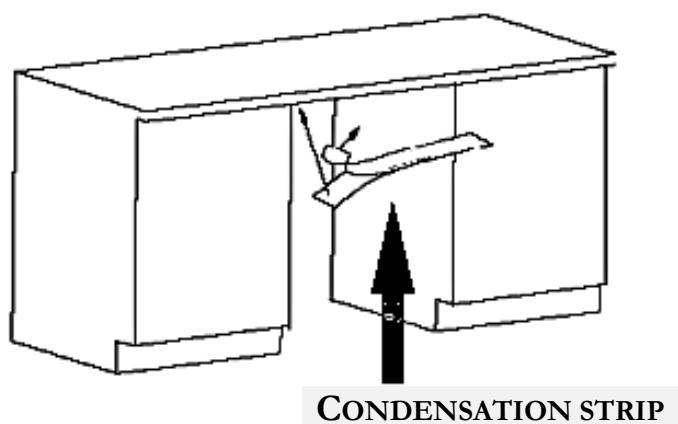
**NOTICE!** Improper installation of the condensation strip may cause damage to the worktop.
