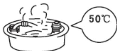
5. Pour warm water (2 - 3 litres / approx. 50 °C) into the drum and wait approx. 10 minutes (s. fig. below).
