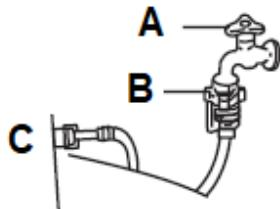
4. Remove the hose and immerse it in warm water (approx. 50 °C / s. fig. below).
