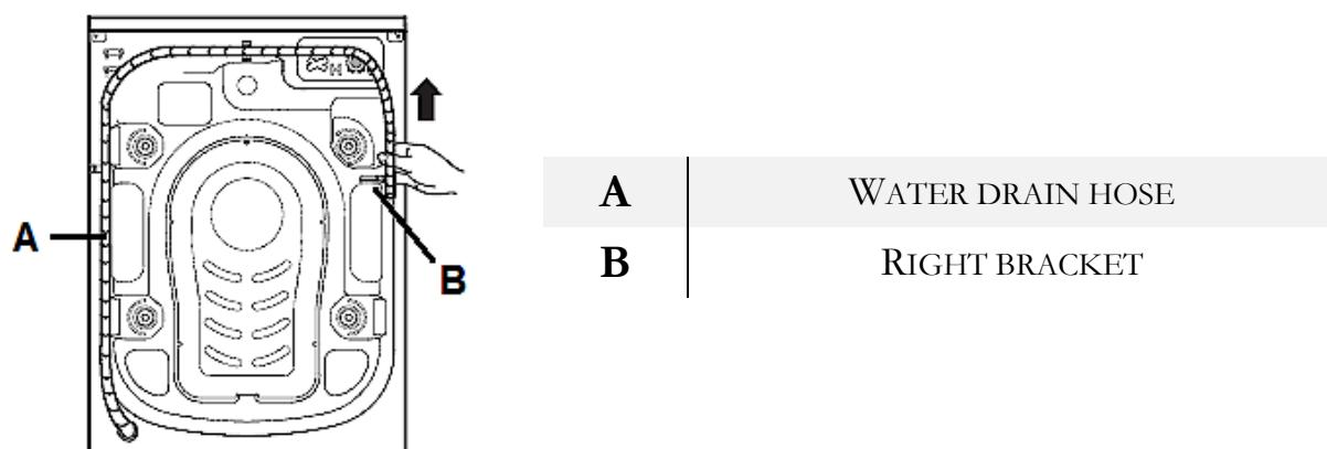
**NOTICE!** If the appliance is out of operation, fix the water drain hose (A) on the back of the appliance using the right bracket (B): s. fig. above. **Do not remove the brackets!**
