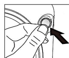
4. Insert the four provided caps into the screw holes (s. fig. on the right / note the direction of the arrow).
