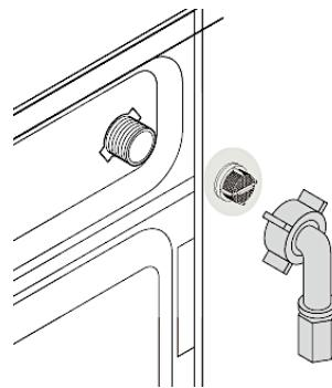
7. Clean the filter using some water and a toothbrush (s. fig. on the right).
