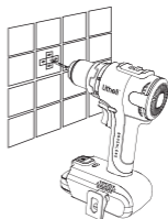
Drilling in tiles without skidding
