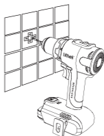
Drilling in tiles without skidding
