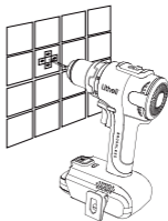
Drilling in tiles without skidding
