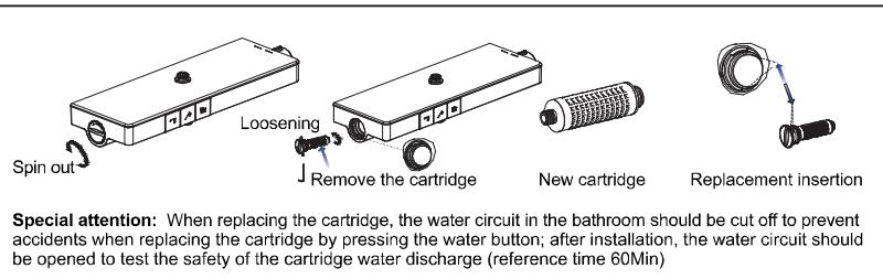
**Special attention:** When replacing the cartridge, the water circuit in the bathroom should be cut off to prevent accidents when replacing the cartridge by pressing the water button; after installation, the water circuit should be opened to test the safety of the cartridge water discharge (reference time 60Min)
