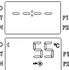
**Turning the appliance off:** simply press the ON/OFF button to turn the water heater off, only "OFF" appears on the display. The protection against corrosion is still ensured, while the product will automatically ensure that the temperature of the water in the tank does not fall below 5°C.
