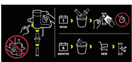
There is a label on the pre-filter of the device that describes how to clean/replace the pre-filter and fine filter:
