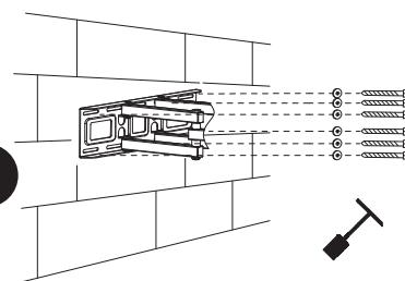
Attach the Part A to the wall using the supplied screws or your own suitable screws, there are long holes to adjust the holder perfectly.
