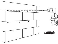
Drill holes with a 10mm Stone drill, use Concrete Anchor(D)
