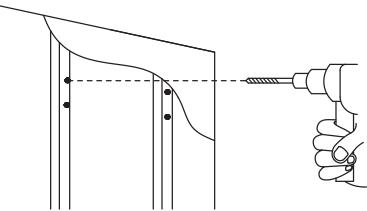
Drill holes with a 4.5mm wood drill.
