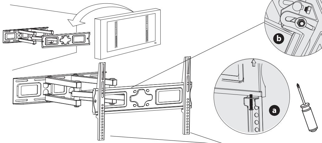
Hook the TV to the wall plate. For additional Security, tighten the screws(a). Tighten or loosen the screw(b) to make the tilt happen.
