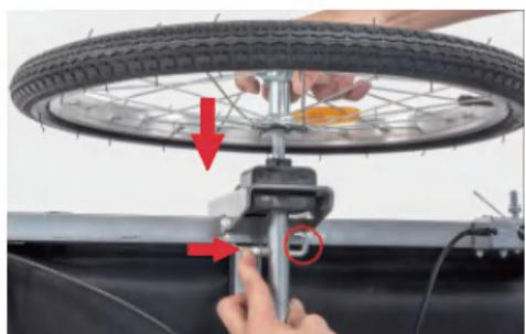
**2. Insert the wheel with axle into the mounting hole on the below crossbar 2 side of the Cabin Frame. Finally release the spring buckle to fix the wheel. Install the 2 wheels into the 2 sides of the frame in the same way.**
