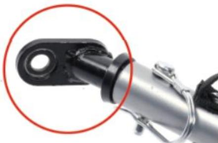
**1.**The head connector part of the long bent rod with the buckles trap is designed with a fixed pin for easy connection to the bicycle.
