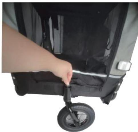
**1. Insert the rod of Y-shaped bracket with Front wheel underside plastic cover into the front mounting hole of fixed on the Cabin frame.**
