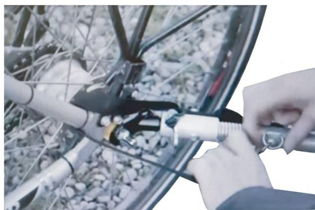
**2.**You can fix attach the head connector part to the rear end of the bike, with a pin for quick attachment or detachment of the trailer.
