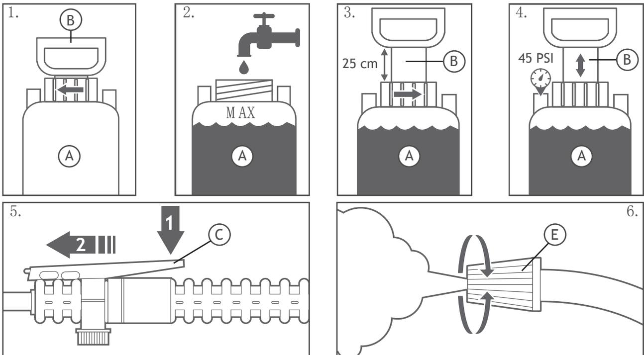
1. Simply unscrew the pump handle (B) counter-clockwise taking care not to damage it.
