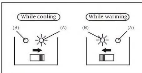
If you want to set an increased energy efficiency and a limited cooling capacity for the cooler unit. Use the cooler's ECO mode.
