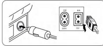
AC: Insert the end of the AC power cord "13" into the AC socket corresponding to the refrigerator, and plug the other end into the power socket.
