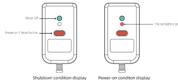
After the electric towel rack is powered on, please first press the test button (green) to power off, and then press the reset button (red) to power on.
