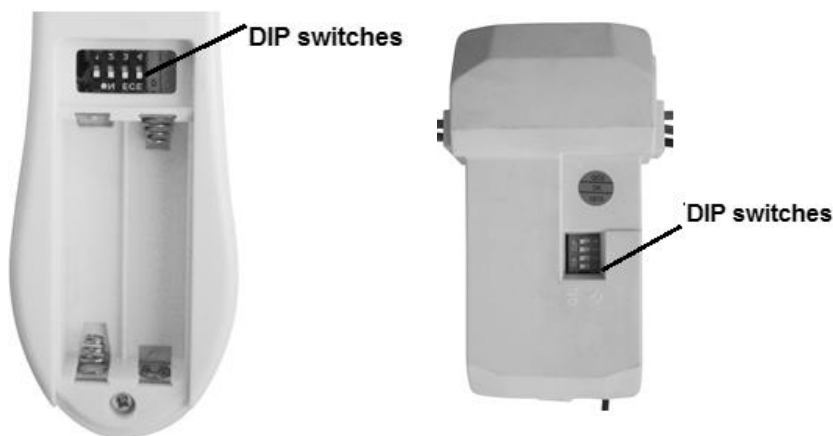
Fig. 8 Remote battery compartment
