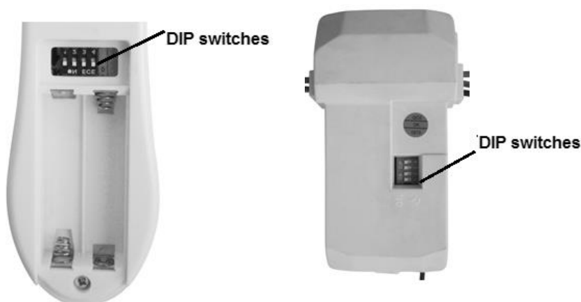
Fig. 8 Remote battery compartment
