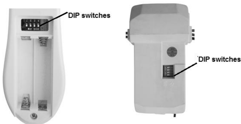
Fig. 8 Remote battery compartment
