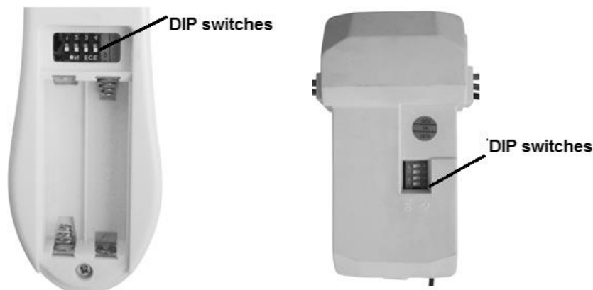
Fig. 8 Remote battery compartment
