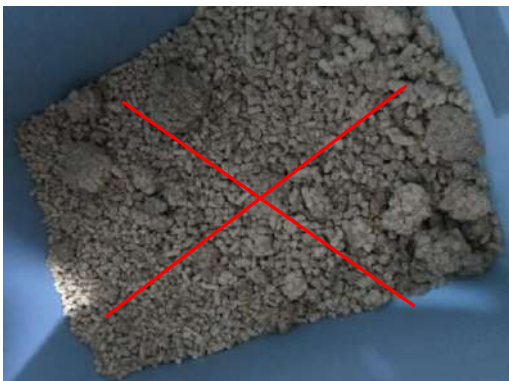
Agglomeration of poor-quality pellets
