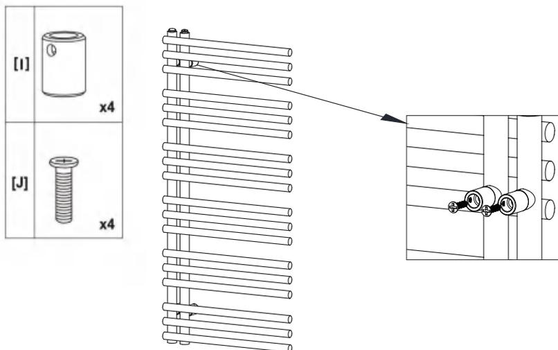
**Step 4:** Mount the radiator to the wall and tighten the Small Screws H in the brackets.
