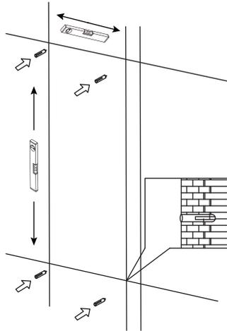
Mark the position of the screws on the wall, then drill four holes accordingly and tap the number F on the wall.
