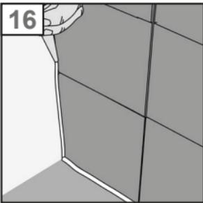
16. Finally, use a suitable silicon to cover the connecting joints between the wall/floor and the glass bricks.
