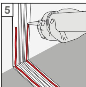
5. Carry on applying the adhesive to the wall profiles, only up to the height of one brick (one row).
