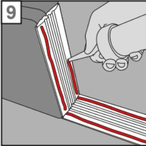
9. Apply more adhesive to the short profile stuck to the glass brick.
