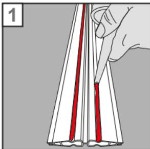
1. Installing floor profiles: apply a 5-6mm thick stripe of glue on the two indentations on the profile.
