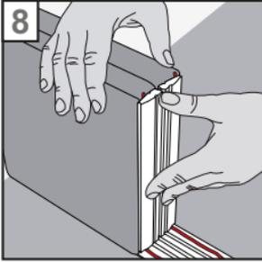
8. Vertically stick the profile onto the side of the glass brick and make sure that you meet the existing long profile below to avoid sticking up into where the next long profile needs to sit.
