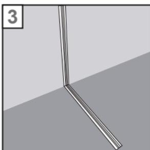
3. Carry on with this process with the wall profile(s). Make sure that the two sets of profiles are at a 90° angle.
