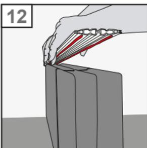
12. Now apply adhesive to the centre of the smooth side of a long profile. Place this profile upside down on the already installed row of bricks. Press on the profile a little to make sure the glue will properly stick onto the row of bricks below.
