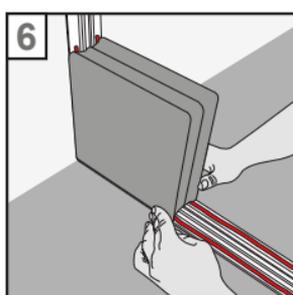
6. Place the first glass brick on the profile; start at the wall. When positioned correctly, the glass brick should sink down a little. Try to carefully lift the brick up a little to make sure that the glue is sticking.
