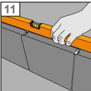
11. Once the first row has been installed, check the alignment. You can adjust as necessary if the glue hasn't dried yet.
