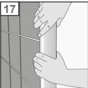
17. If you didn't use end bricks, you can cover the connecting ends of the wall with end profiles. Available from us in: aluminium satin, aluminium white, brushed stainless steel and polished stainless steel.
