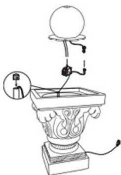
2. Connect the cord of the pump to the transformer. Then, plug the transformer into a grounded electrical outlet.
