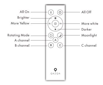
Note: The Light Fitting & the Remote Control have been paired "A channel" at the factory. If the remote control is not working you may need to action the following pairing process.
