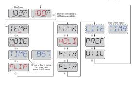
Waiting a few seconds in the Main Menu will allow the display to revert to the Main Screen. Most changes are not saved unless Light (i) is pressed. Refer to key above.
