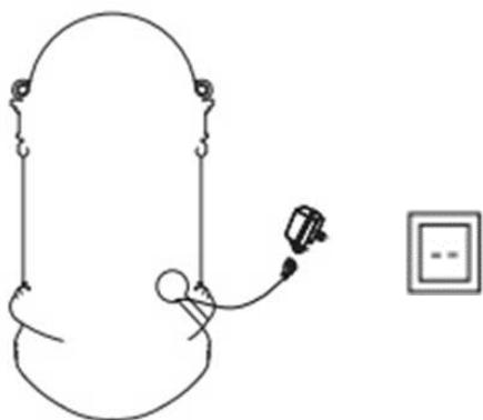
3. Fill the fountain with enough clean water to ensure the pump remains fully submerged during operation. Conduct a test run of the fountain. Adjust the water flow rate on the pump as necessary.
