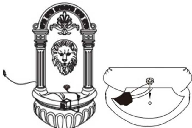
2. Connect the cord of the pump to the transformer, then plug the transformer into a properly grounded outlet.
