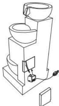
2. Insert the cover in place and plug the pump cord into a properly grounded outlet.
