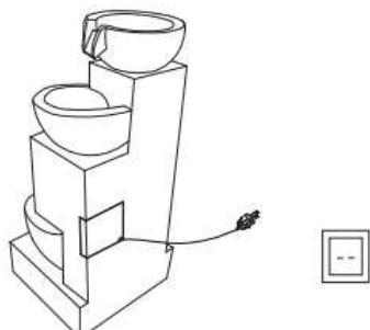
3. Fill the fountain with enough clean water to keep the pump fully submerged during operation.
