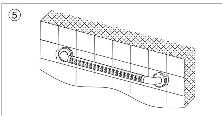
**EN** After confirming that the product is secure and free from looseness, fix the handrail cover in the snap-in position.
