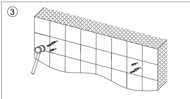
**EN** Place the plastic expansion plug into the drilled hole, inserting it completely into the hole.
