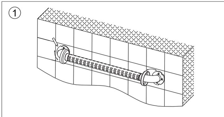
**EN** Unscrew the cover of the handrail, place the handrail on the mounting position and draw the mounting holes on the wall with a pencil, it is recommended to choose 3 symmetrical holes.
