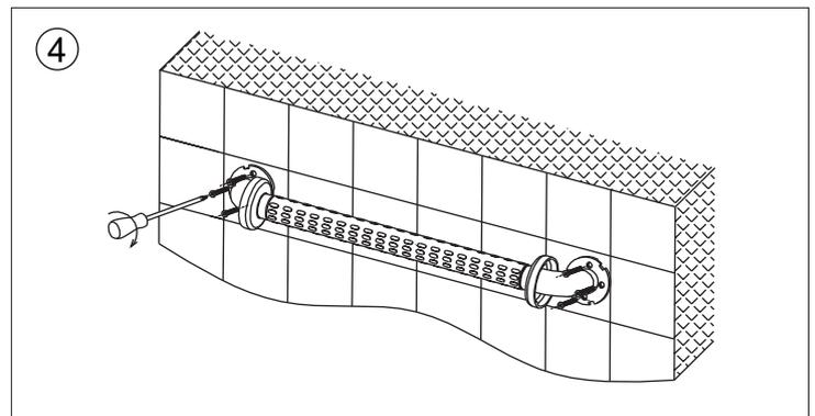
**EN** Place the handrail at the hole and tighten the screw through the base plate with a screwdriver to secure it.
