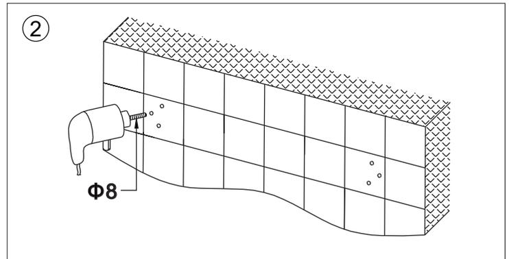
**EN** Drill holes in the marked wall with an impact drill,  $\varnothing 8$  bit is recommended.
