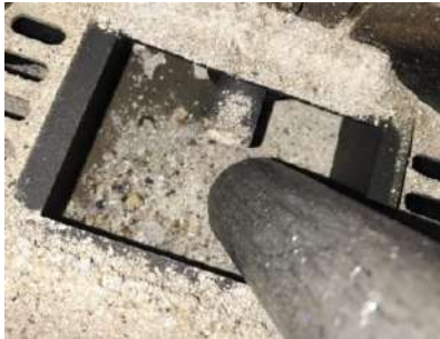
Example of a dirty base
