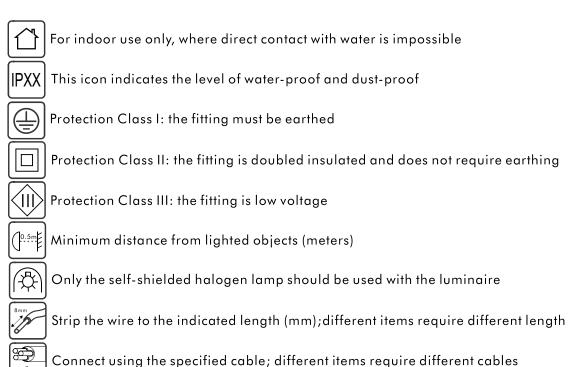
Max.; 50mm GU10 2Max.50W The type of lamp and maximum size and wattage indicated in each lighting unit must not be exceed; different items require different kind of light sources with different bulb icons
